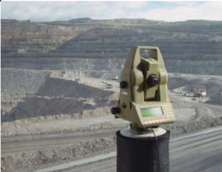
With a large field of view, a single Leica TCA 1800 controlled by ALERT software can monitor multiple extraction areas.
