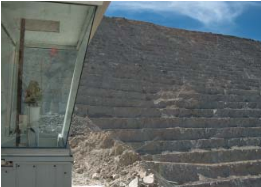
A Leica TCA 1800 keeps a 24/7 watchful eye on the open pit mine to maintain a safe working environment.
