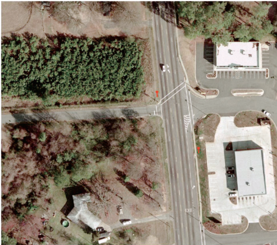
A screen shot showing how the GS50 collected bus stop data lines up with the County's digital ortho photo (0.5-foot pixel resolution)
